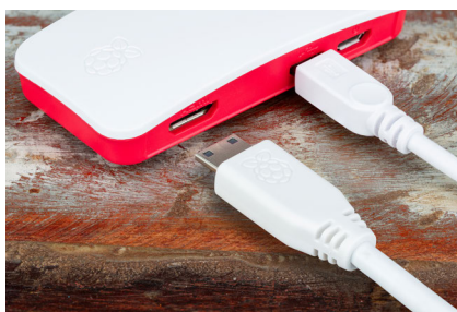
Figure 2-17 Connecting the HDMI cable to a Raspberry Pi Zero
