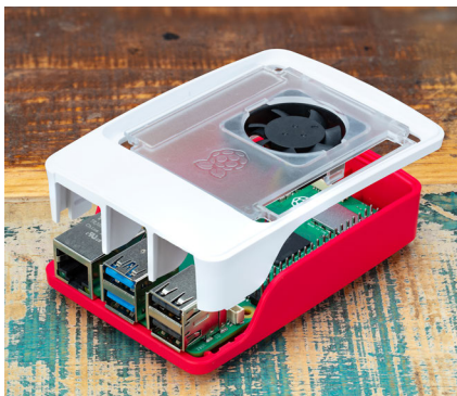
Figure 2-7 Attaching the fan assembly and frame
