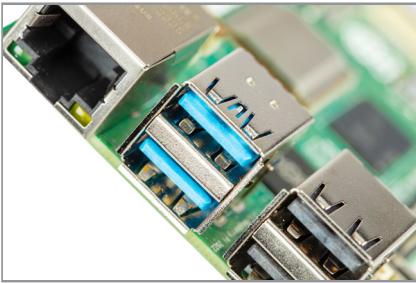
Figure 1-7 Raspberry Pi's USB ports
