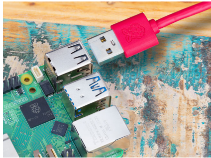
Figure 2-15 Plugging a USB cable into a Raspberry Pi 5
