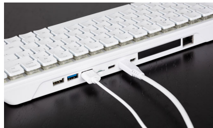
Figure 2-23 Connecting the HDMI cable to a Raspberry Pi 500+
