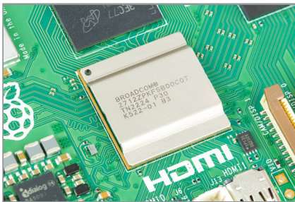
Figure 1-2 Raspberry Pi's system-on-chip (SoC)
