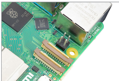
Figure 1-9 Raspberry Pi's Power-over-Ethernet connector
