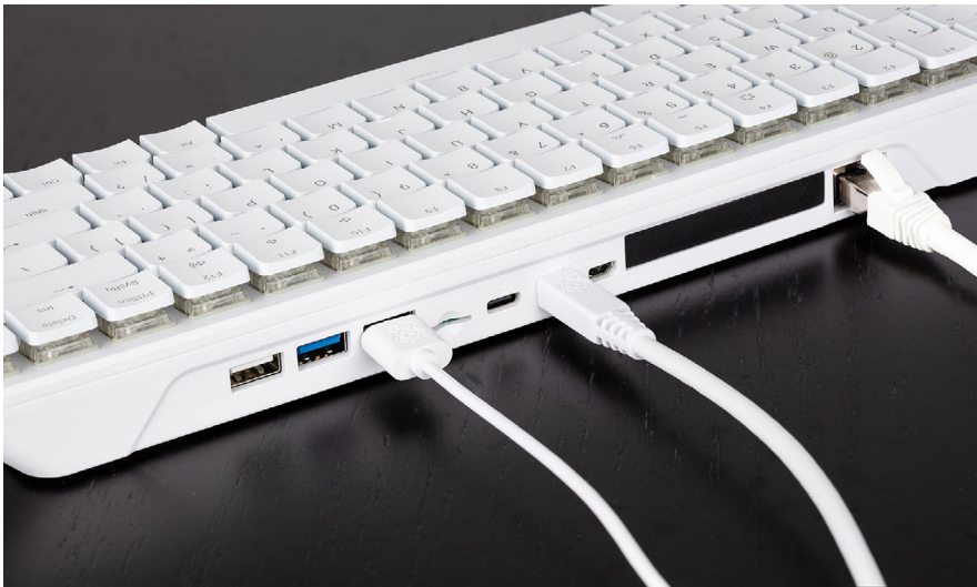
Figure 2-24 Connecting Raspberry Pi 500+ to Ethernet
