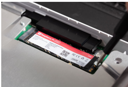
Figure 2-30 Remove the M.2 retaining screw
