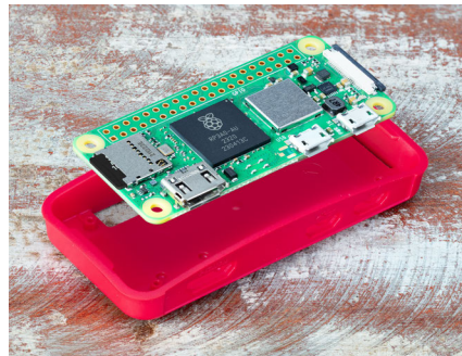
Figure 2-11 Placing the Zero 2 W in its case
