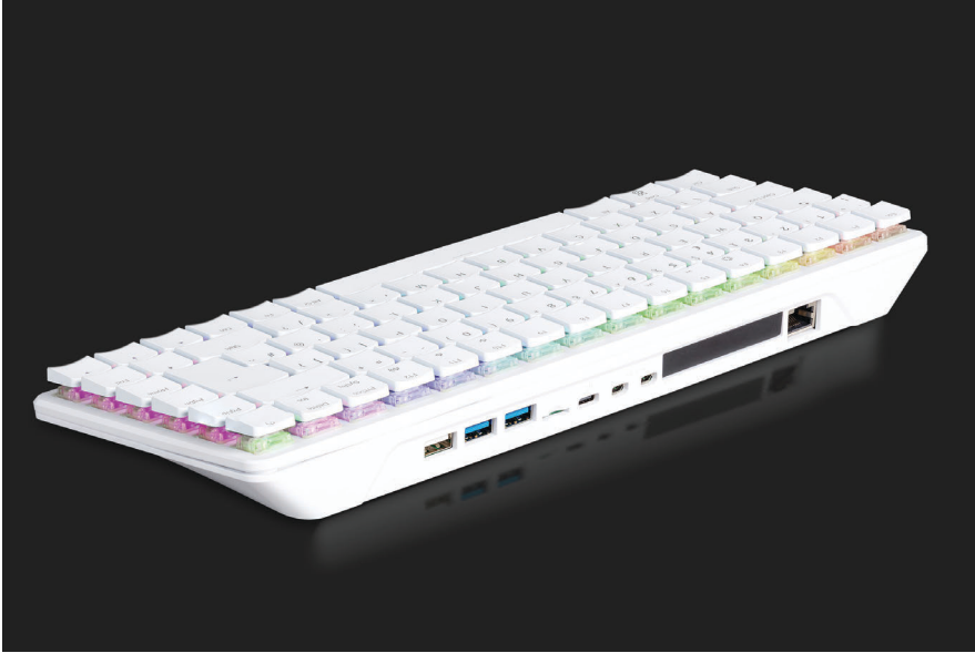
Figure 1-17 Raspberry Pi 500+ has a keyboard in front, ports in the back
