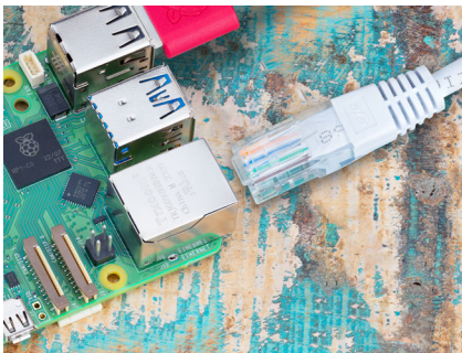
Figure 2-18 Connecting Raspberry Pi 5 to Ethernet
