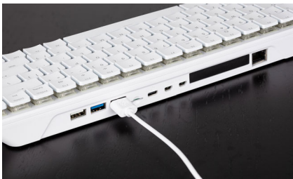
Figure 2-22 Plugging a USB cable into a Raspberry Pi 500+
