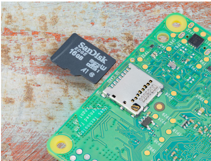
Figure 2-14 Inserting the microSD card
