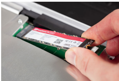
Figure 2-31 Removing the SSD
